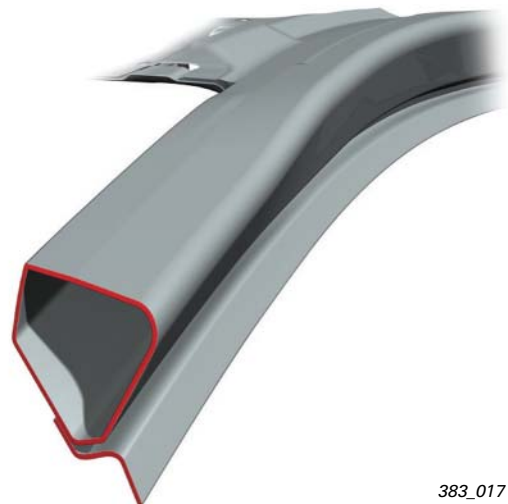
A-post, Audi A8 Single-chamber extruded section
