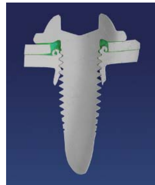
Micrograph of a Flow Drill screw connection
